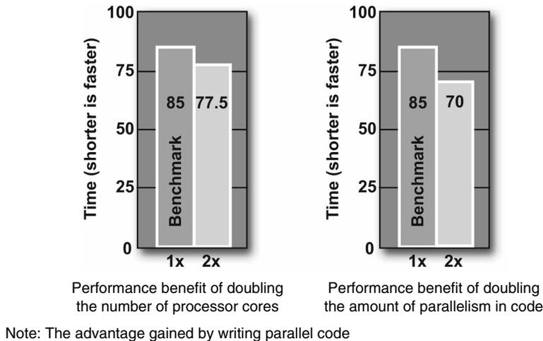
**Figure 1.7** Theoretical Performance Comparison between Increasing Number of CPU Cores versus Increasing Concurrency in Implementation
