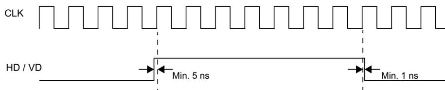
Fig. 6 HD/VD setup timing
