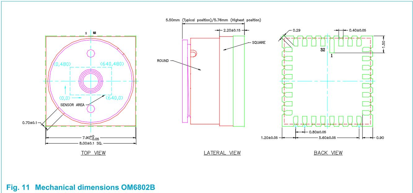
Fig. 11 Mechanical dimensions OM6802B
