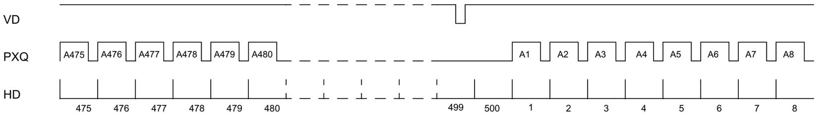
Sub-sampling by 2, QVGA output stream
