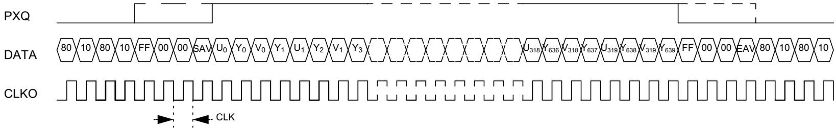
Sub-sampling by 2, QVGA continuous data stream
