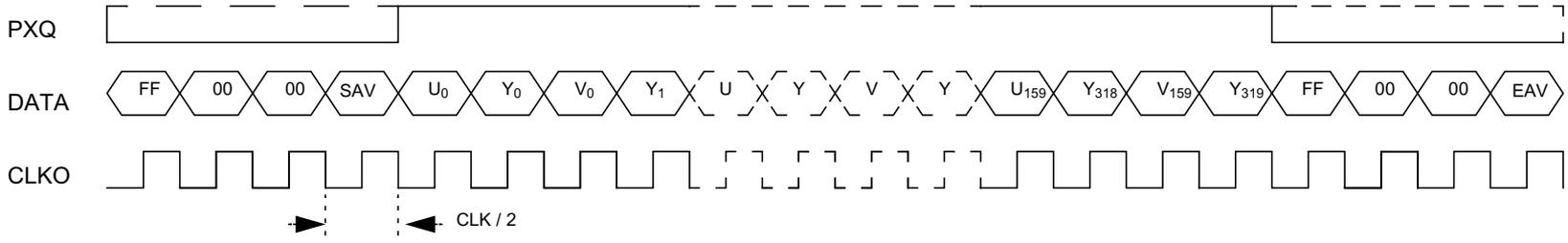
Sub-sampling by 4, QQVGA continuous data stream
