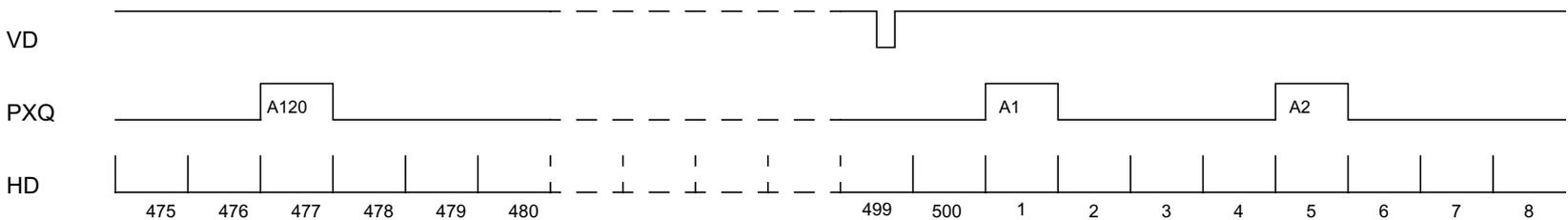
\* Above timing diagrams depict 2 and 4 times sub-sampling. 3 and 5 times subsampling is done in a comparable way.
