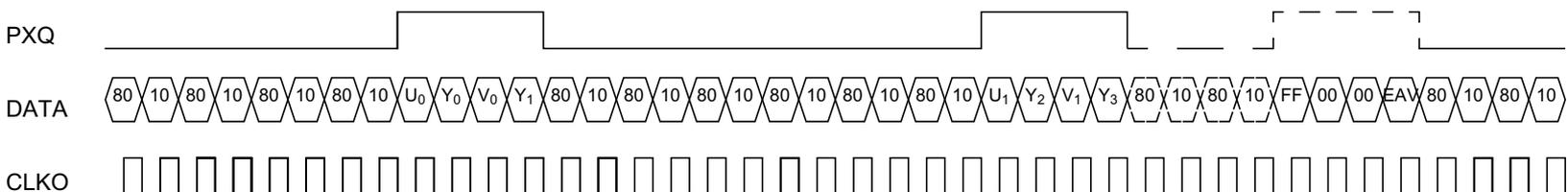
\* Above timing diagrams depict 2 and 4 times sub-sampling. 3 and 5 times subsampling is done in a comparable way.
