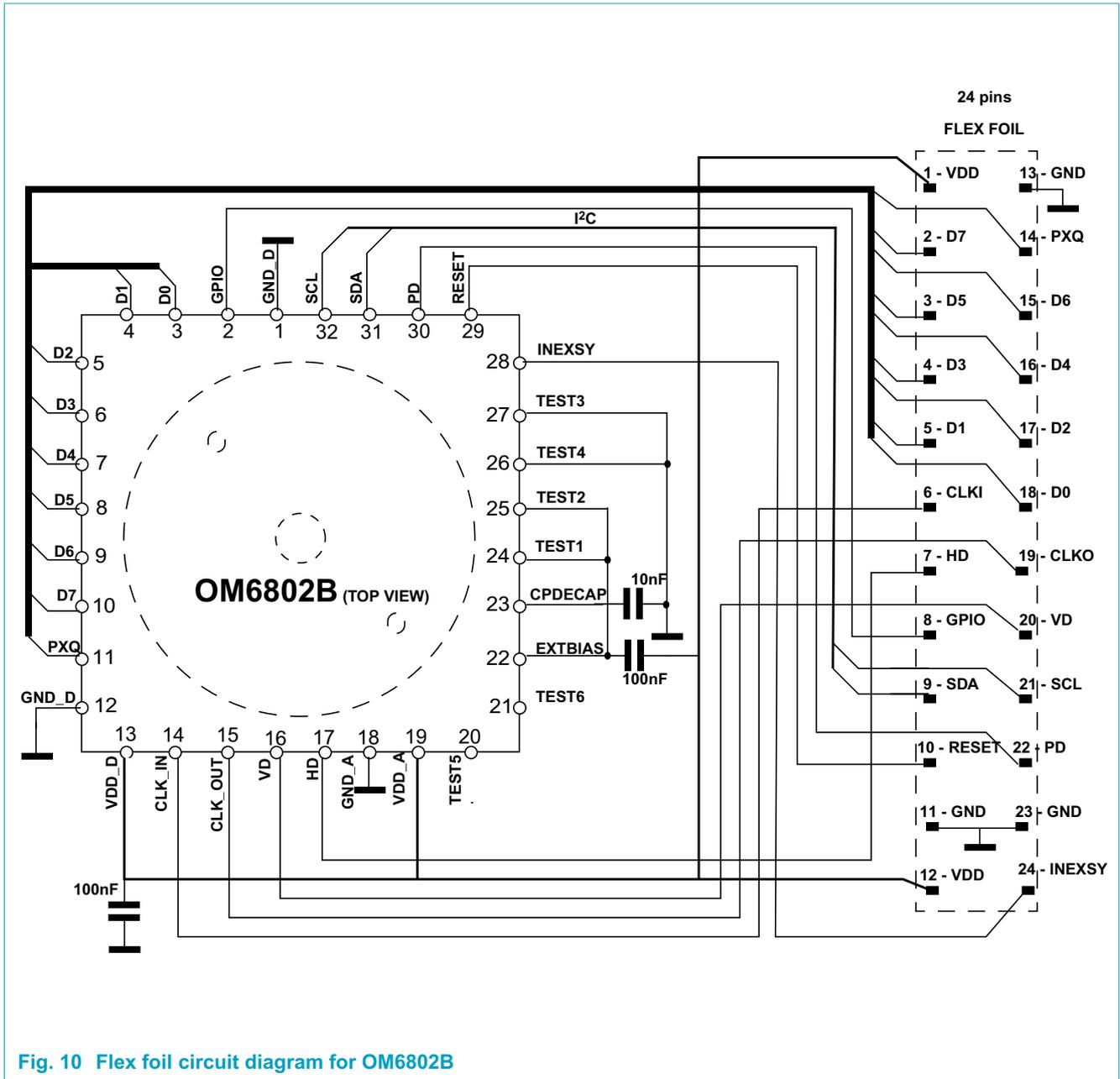
Fig. 10 Flex foil circuit diagram for OM6802B
