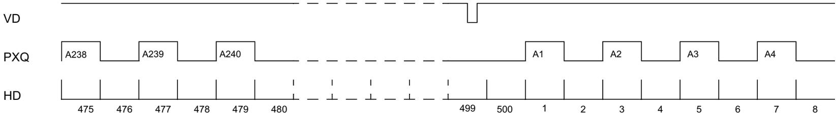
Sub-sampling by 4, QQVGA output stream
