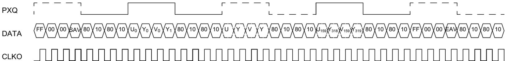
Sub-sampling by 4, QQVGA discontinuous data stream
