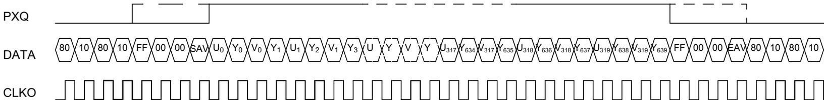
Sub-sampling by 2, QVGA discontinuous data stream
