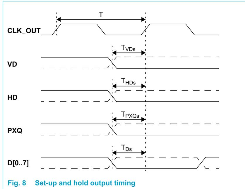
Fig. 8 Set-up and hold output timing
