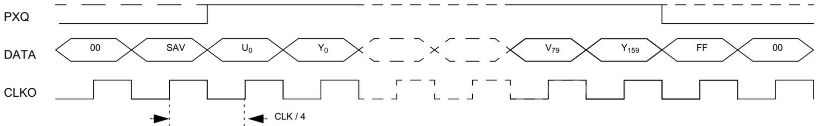
\* Above timing diagrams depict 2 and 4 times sub-sampling. 3 and 5 times subsampling is done in a comparable way.
